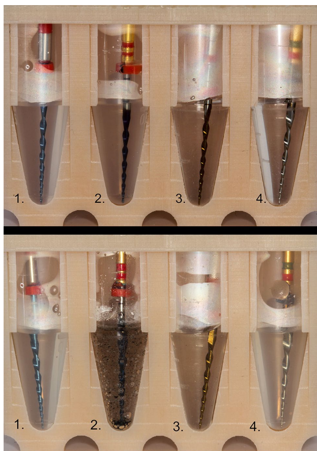
Fig. 3 Immersion of the tested file systems: (1) Reciproc Blue, (2) CC One Blue, (3) EdgeOne R-Utopia, (4) Procodile Q. The top image shows immersion in 60 °C distilled water, while the bottom image depicts immersion in 60 °C sodium hypochlorite (NaOCl). Noticeable dissolution, turbidity and chemical reactions are evident in (2) CC One Blue, indicating an interaction between NaOCl and the nano-coating
